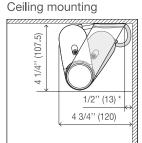
\*This is the minimum dimension to prevent interference with the walls or ceilings. Make sure to install with a distance of the described length or more from the walls or ceilings.
