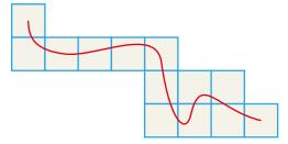
Selecting sections by "Pen" tool Sections through which the pen passed are selected.
