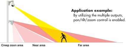
Note: The ambient temperature, installation height and mounting angle may change the detection ranges for each of the areas.
