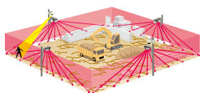
Vertical detection area example
