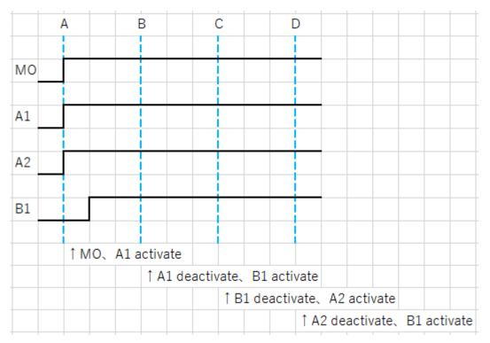
Since "A1" and "A2" were detected at time "A", "A1" and "MO" with high priority are activated. "Latest" was "A1". After that, "B1" was detected, so "A1" was deactivated and "B1" was activated at time "B". "Latest" was "B1". "A2" that was not notified was notified at time "C". Since "A2" notified at time "C" was not "Latest", reactivate "B1" which is "Latest" at time "D".
