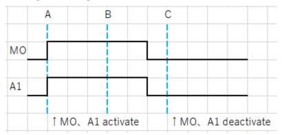
Since "A1" was detected at time "A", "MO" and "A1" were notified activation. Since "A1" was cleared between times "B" and "C", deactivation was notified at time "C".
