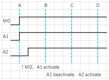
Since "A1" was detected at time "A", "A1" was activated. "Latest" was "A1". After that, "A2" was detected, so "A1" was deactivated and "A2" was activated at time "B". "Latest" was "A2".
