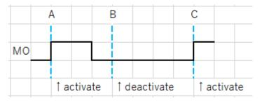
Since "MO" was detected at time "A", the "Notification timing" is set to time "A". After that, "MO" was cleared, so it will be deactivated at time "B". Since all the events have been cleared, the "Notification timing" after time "B" will be undefined. After that, "MO" was detected at time "C", so the "Notification timing" will set again from this point.
