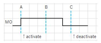
The blue dotted line indicates the notification timing. MO was detected at time "A". At this time, "activate" is issued to the device. Since the event has not changed at time B, nothing is notified. MO was cleared before time "C". The notification function issues "deactivate" at time "C".
