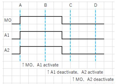
"A1" and "A2" were detected at time "A". According to priority, "MO" and "A1" were activated at time "A". At time "B", "A1" was deactivated and then "A2" was activated. After that, "A1" and "A2" were cleared. Therefore, "MO" and "A2" were deactivated at time "C".
