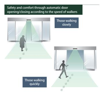
VVS-1 is able to accurately recognize the speed at which someone approaches the automatic doors, allowing for faster or slower-than-usual openings for those walking. This ensures the optimum open timing for pedestrians and allows for safe, comfortable passage through the doors.
