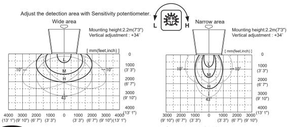
NOTE When the sensor is mounted at higher than 3.0m, set the Sensitivity to "H (high)".
